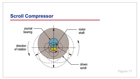
The center of the scroll journal bearing and the center of the motor shaft are offset. This offset imparts an orbiting motion to the driven scroll. Rotation of the motor shaft causes the scroll to orbit—not rotate—about the shaft center.
